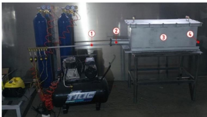
Fig. 1. Laboratory georeactor for UCG study - 1. Injection well, 2. Ignition window, 3. Gasification chamber, 4. Production well.
