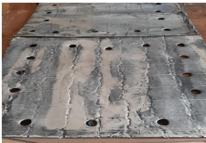
Fig. 1. 0.8 mm steel wire reinforced composite. Pitch (distance) - 50 mm.
