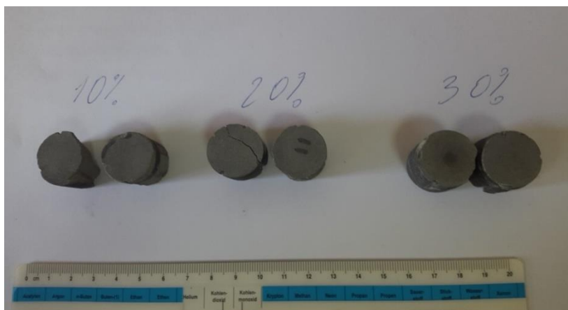
Fig. 1. Samples containing different percentage of Aluminum powder compacted by explosive technology
