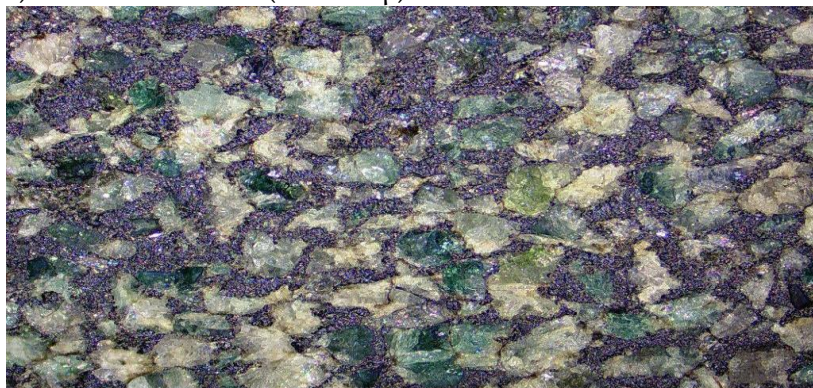
Fig. 2. The microstructures of samples from explosive compacted silicium carbide and aluminum charge mixture, in size 120-150 \mu
