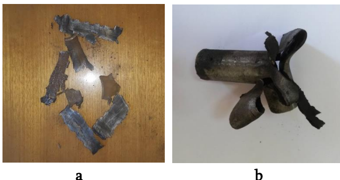
Fig. 4 Typical images of steel tube fragmentation (a) and deformation (b) after explosion
