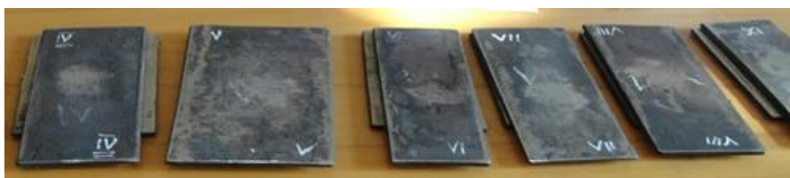
Fig. 4. Explosive-welded steel plates of different hardness
